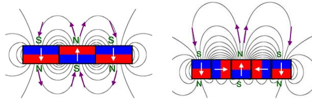
Figure 18. Halbach array in the rectangular form [23]
