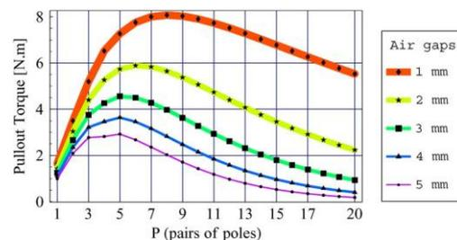
**Figure 2.** Torque versus the number of pole pairs [2]
