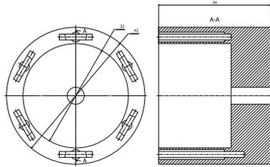
Figure 9. Radial, female 6 poles (arrangement 5)
