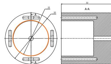
Figure 5. Radial, female 4 poles (arrangement 1)
