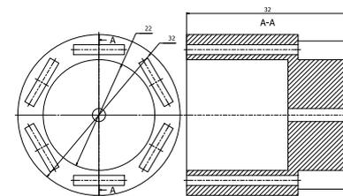
Figure 6. Radial, female 6 poles (arrangement 2)
