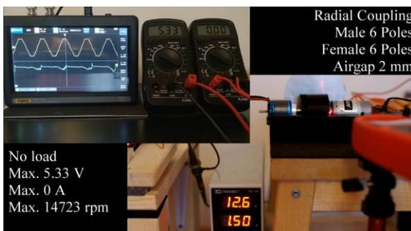
Figure 17. Screenshot of the experiment for arrangement 5
