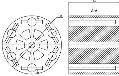
Figure 8. Radial, male 6 poles (arrangement 5)
