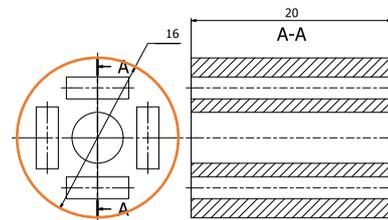
Figure 4. Radial, male 4 poles (arrangement 1 and 2)
