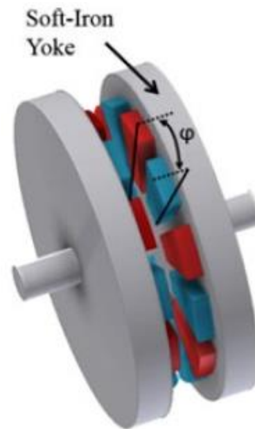
Figure 3. Schema of a Disc Coupling [2]
