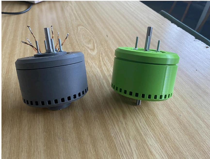
Figure 3: Two variations of the main open-source motor model constructed using 3D printing: the left model is made entirely of iron-embedded PLA, while the right model uses iron-embedded PLA only for the core
